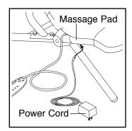
Next, it is recommended that you disconnect the wire harness on the hand control from the wire harness on the massage pad. To disconnect the wire harnesses, first press down the indicated small latch.
